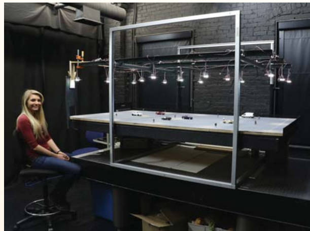
A Lighting Research Center student with the parking lot mockup designed for the study.
