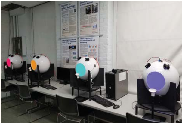
Diffused light was delivered through the front opening (8 in. diameter) of a custom-built sphere (16 in. diameter) fitted with high-power LEDs.
