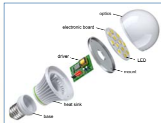
Exploded view of an LED lamp
