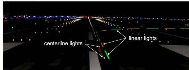
Cockpit simulator presentation of a right 30° turn with 32-ft linear elements and 50-ft spacing
