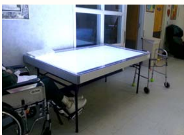
Figure 1. An LED edge-lit television was inserted in a table frame to deliver light to ADRD patients.
