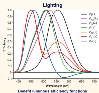
The solution is a family of benefit efficiency functions, each characterizing the spectral sensitivity of a different visual or non-visual channel, to determine which light source provides the greatest benefit for a given design
