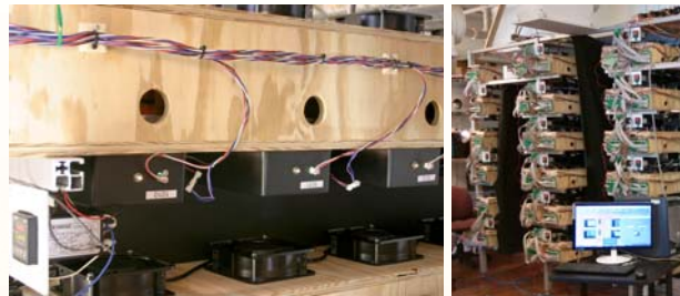
Individual test chamber design with five product samples in each box. The setup controls the lighting system temperature and on-off cycles accurately while continuously monitoring the light output, LED system temperature, and power input of each product. Furthermore, the spectral power distribution of each product is measured at regular intervals. Racks house the 270 LED product samples and the computer controlled data acquisition system.
