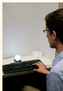
(left) A subject views the flickering light source as displayed for human factors testing of the metric. (right) Relationship between flicker detection probability and the metric value.
