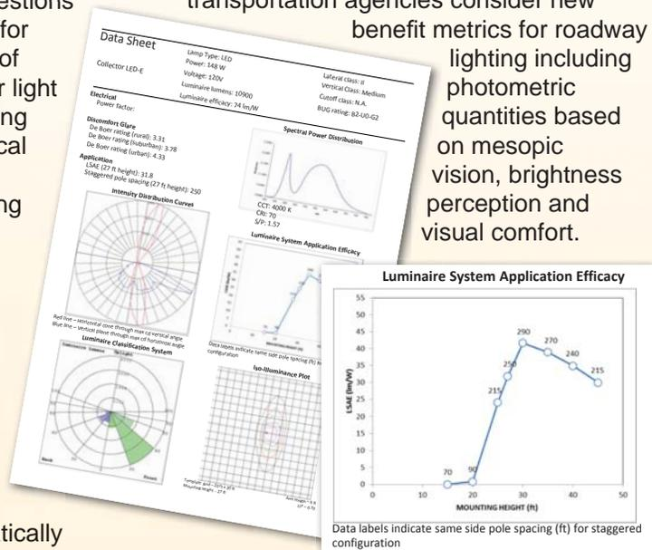
The data sheets developed by the LRC show how pole spacing (data labels) and luminaire system application efficacy, or LSAE (vertical axis), are impacted by mounting height (vertical axis).
