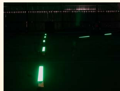
Linear lighting elements were evaluated in a full-scale, darkened, indoor area to simulate airfield delineation conditions.
