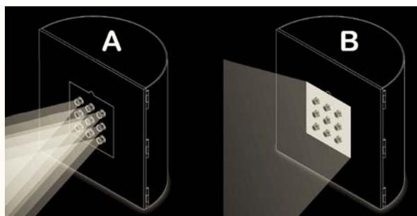
Illustration of the LED apparatus showing the LED array glare source (A) and the luminous surround mode (B).
