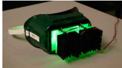
Light mask used in the two studies to deliver individualized doses of 527 nm, “green” light.
