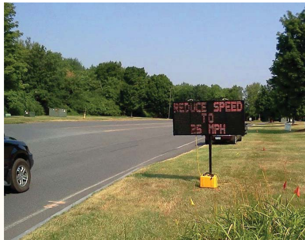
Speed-dependent signs helped reduce speed variance in this field experiment.
