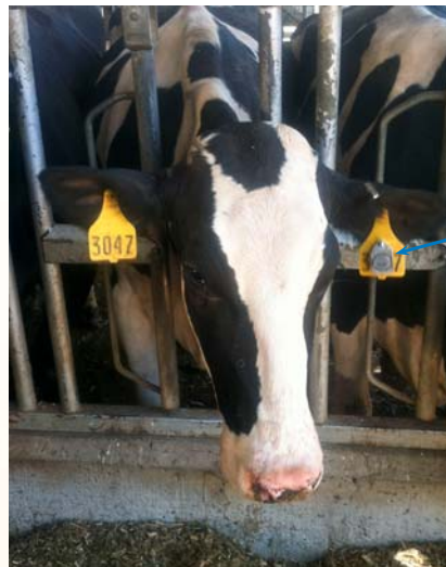
A Daysimeter attached to the cow's ear tag continuously records the light level in close proximity to the cow's eye. The Daysimeter also measures movement of the cow (i.e., activity level), which, together with light exposure, is used to measure circadian entrainment.
