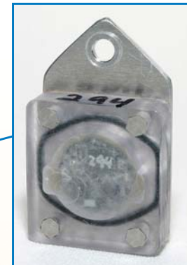
The Daysimeter package with special waterproof housing designed for use with cows
