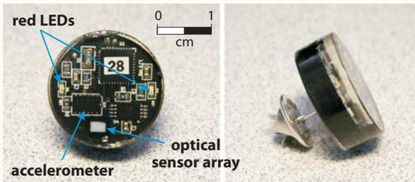
The Dimesimeter is calibrated in terms of the spectral sensitivities of the visual and the circadian systems. Light sensing is performed with an integrated circuit (IC) sensor array that includes optical filters for three measurement channels: red (R), green (G), and blue (B). A monolithic IC accelerometer measures accelerations in each of three planes. It can be deployed for subsequent data download and analysis for continuous usage for up to a month.
