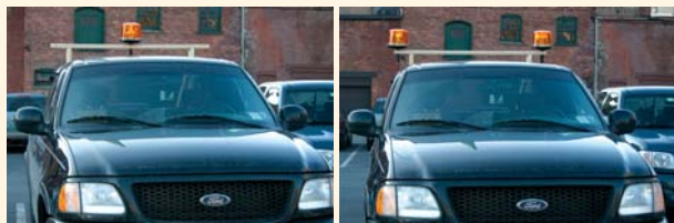
Warning beacon lights mounted on the test truck—single configuration, left, and pair configuration, right.
