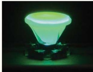
Above: An SPE LED package with a green phosphor when excited by a blue LED excitation light source.
