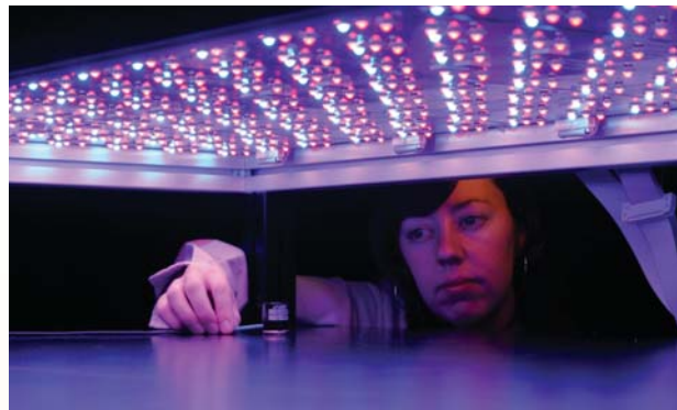
An LRC research technician measures illuminance levels of the prototype lighting system prior to field evaluations.
