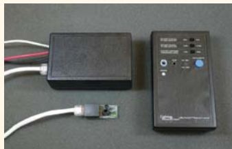
The elements of the DaySwitch (clockwise from upper left): control module, remote commissioning device, sensor module.
