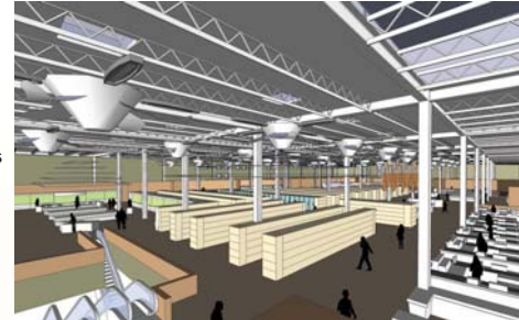
The daylighting scheme for this large-scale food supplier uses roof monitors, skylights, and an integrated skylight system that incorporates the company's graphics into the diffuser design.
