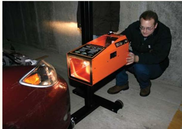
LRC researcher adjusts headlamp aim measurement equipment.
