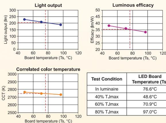
Data for one sample commercial light engine are plotted above. The data points show the performance at each of the three tested board temperatures. The vertical dashed line shows the board temperature measured with the light engine placed inside a decorative pendant luminaire, 76.6°C, and the horizontal dashed line shows the light engine's performance at this temperature.
