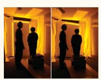
dim lighting conditions. The novel night-light system was built using three linear arrays of amber light-emitting diodes (LEDs) and was attached to a door frame.
