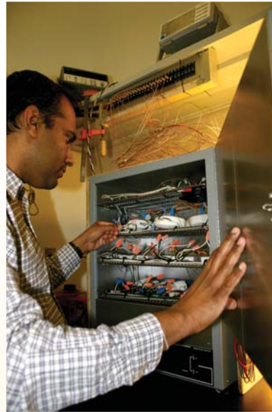
Ballasts were operated inside a thermal chamber during the ACTV stress test. The ballasts operated fluorescent lamps placed outside the chamber.
