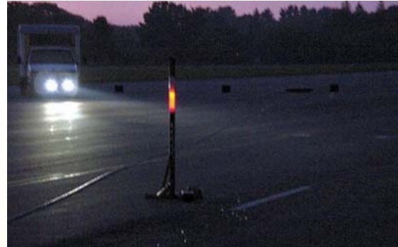
A view of the experimental setup. Subjects looked toward a lighted array and responded to flashing signals from targets located in their peripheral field of view. LRC researchers recorded subject response times for each oncoming headlamp intensity, color, and size.
