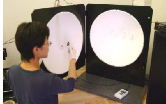
A white LED is placed inside an integrating sphere for light output and spectrum measurements.
