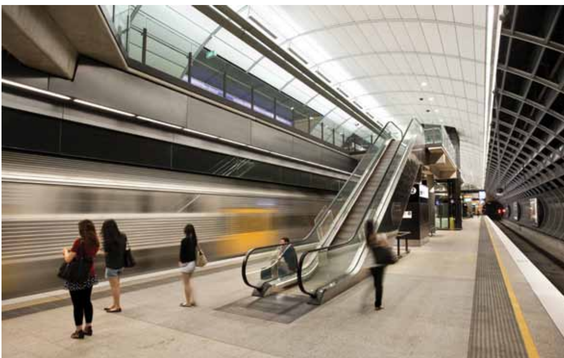
Warmer colour temperatures create a feeling of relaxation in passenger waiting areas. Photography by Brett Winstone, image courtesy of PointOfView.
