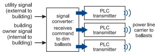
Until now, controlling fluorescent lighting loads required customized solutions with expensive hardware and installation. The load-shedding ballast avoids the cost and complexity associated with traditional dimming methods. These new components are specifically designed for load management and energy efficiency.
