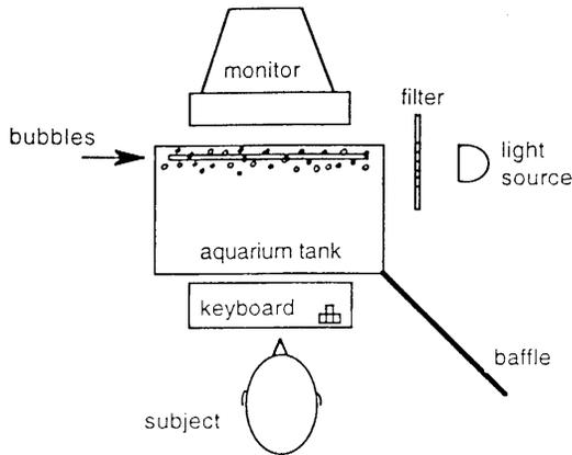
Figure 3. Plan view sketch of experimental apparatus.
