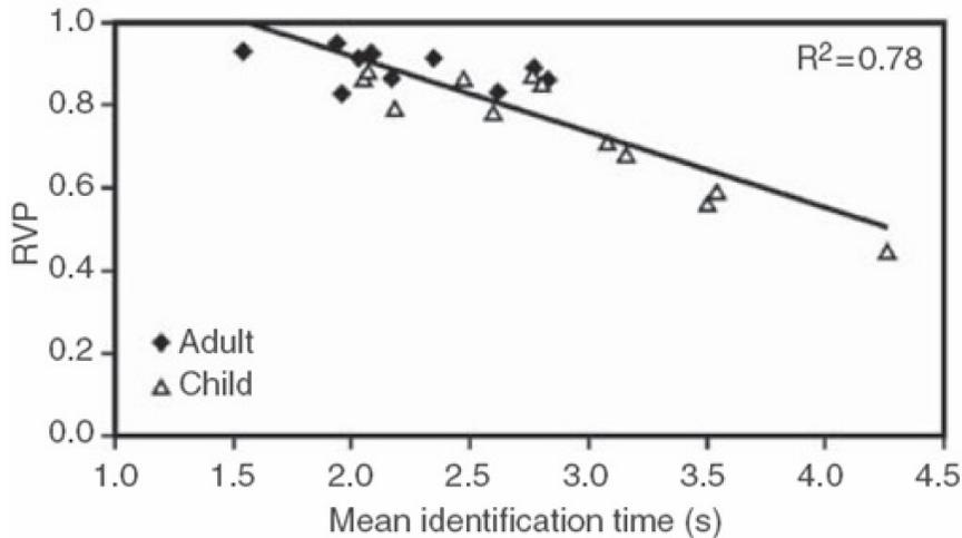
Figure 2. Calculated RVP values and pedestrian identification times measured under different crosswalk fixed lighting conditions, for simulated adult-and child-sized pedestrians.<sup>19</sup>
