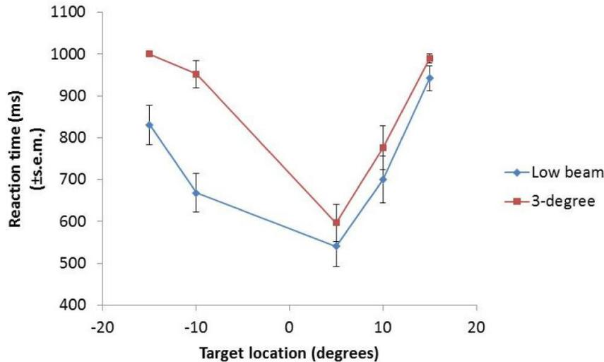
Figure 5. Average reaction times to the onset of targets in the presence of low beam headlights and in the presence of the prototype ADB system evaluated by Skinner and Bullough.<sup>8</sup>
