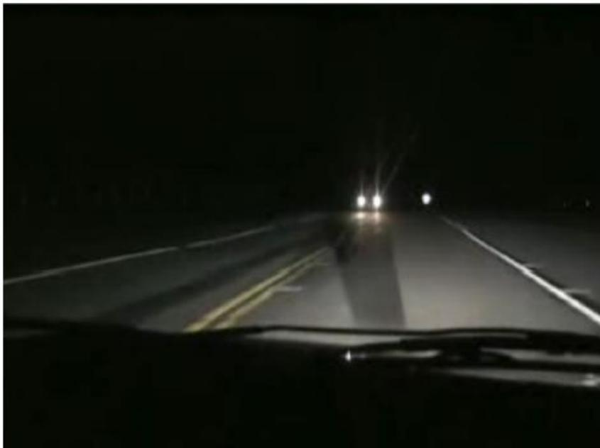
*Figure 1. Driver's view of a prototype adaptive driving beam system with reduced light output toward an oncoming vehicle.<sup>8</sup>*
