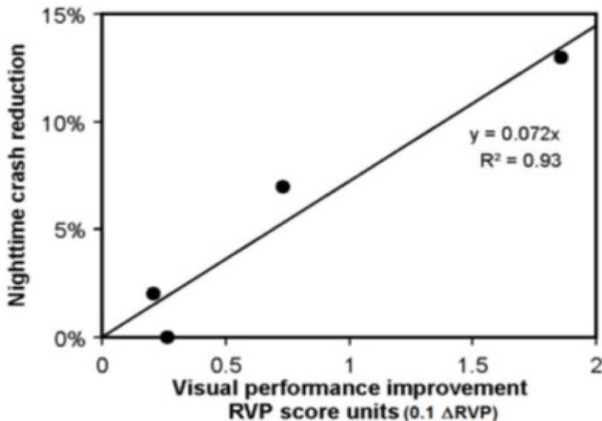
Figure 3. The relationship between RVP improvements from lighting and nighttime crash reductions for different intersection types.<sup>21</sup>
