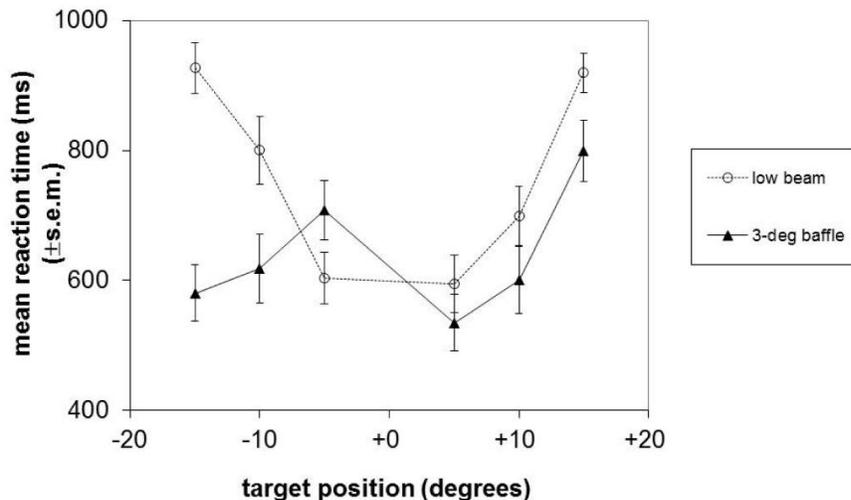
Figure 4. Average reaction times to targets positioned at various angular locations under low beam and under the prototype ADB headlight system.<sup>8</sup>
