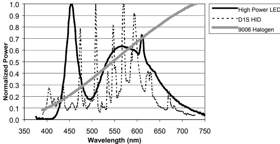
**Figure 7.** Spectral distributions of a high flux LED compared to that of a 9006 halogen lamp and a D1S HID lamp.
