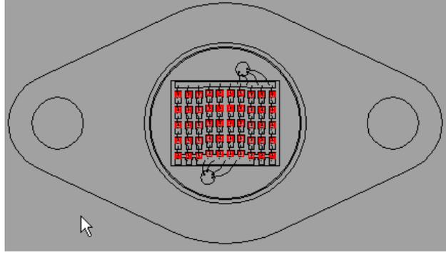
**Figure 2.** High flux LED source with 50 emitters and a total flux output of 42 lm.
