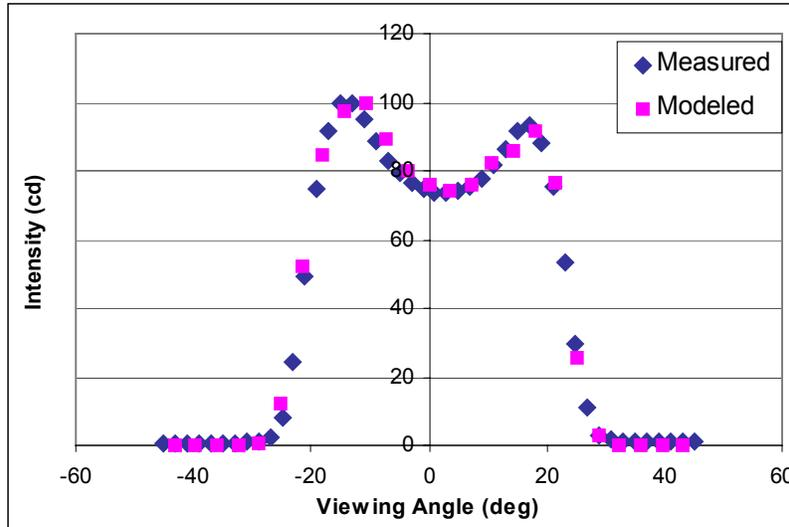
Figure 5. Measured and computer simulated intensity distribution for the example high flux LED with 30° CPC reflector.
