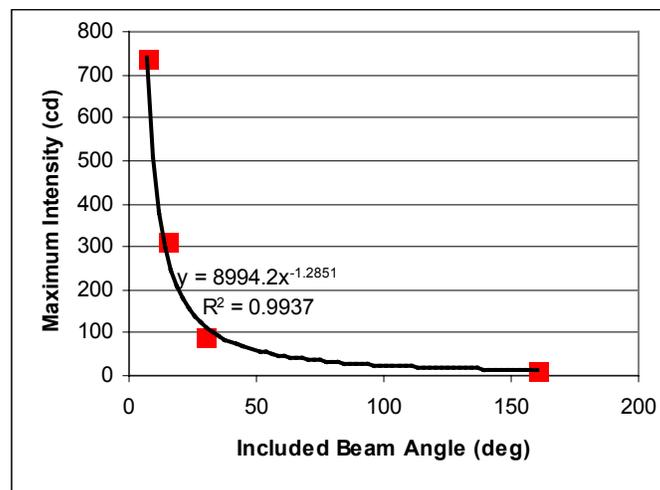
Figure 6. Maximum beam intensity as a function of designed CPC beam angle for the example high flux LED.
