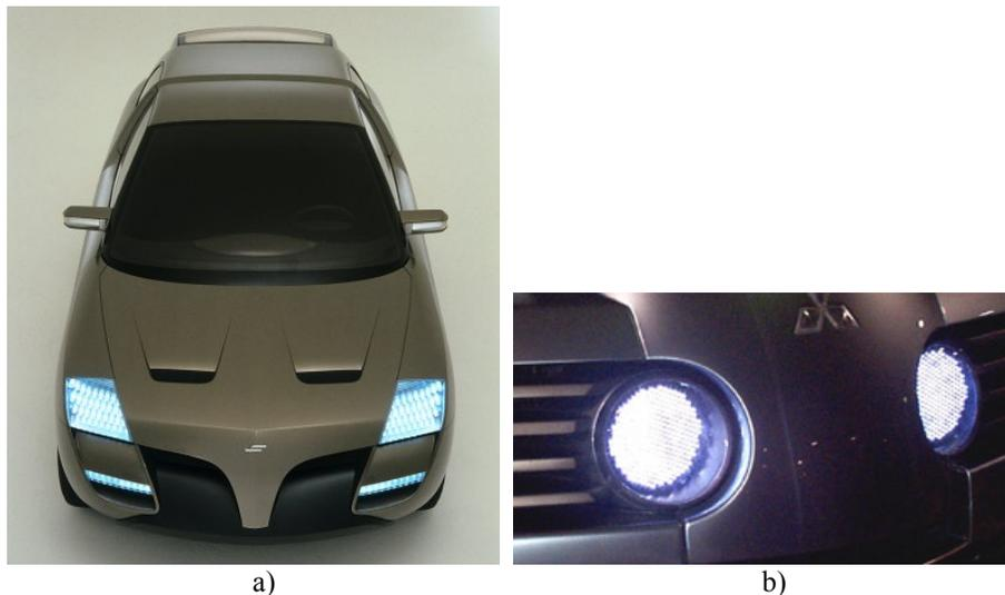
**Figure 1.** White LED forward lighting on concept vehicles. a) A high flux based LED forward lighting system on Fioravanti Yak concept vehicle. b) A 5 mm array based LED forward lighting system on a Mitsubishi SSU concept vehicle.
