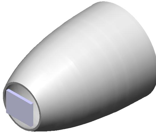
**Figure 4.** Modeled CPC reflector and LED source for the  $30^\circ$  beam angle case.
