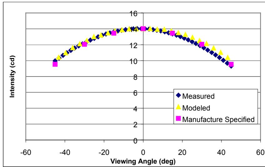
**Figure 3.** Measured, specified and modeled intensity distribution of the example high flux LED source.
