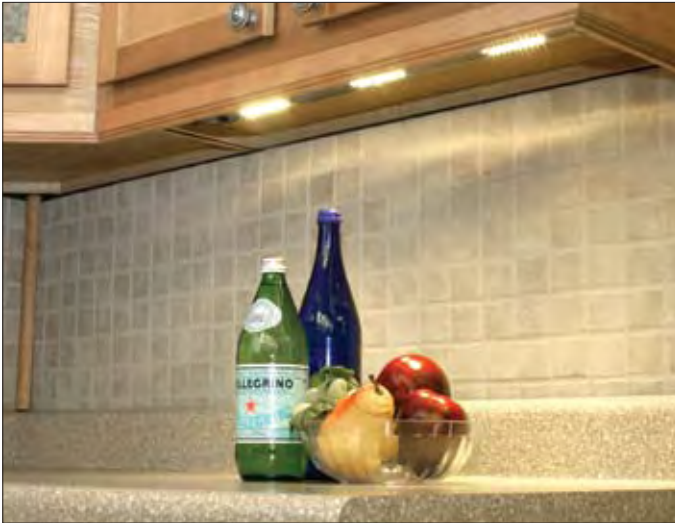
An LED-based under-cabinet fixture. ASSIST recommends that the application efficacy is calculated as the total lumens on the task plane, divided by the total fixture input power.
