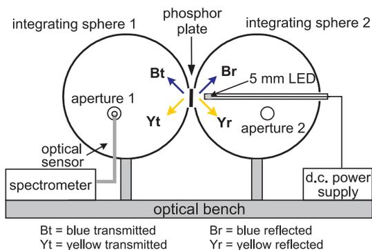
**Figure 1** (online colour at: www.pss-rapid.com) Experimental setup used for measuring the light transmitted and reflected from the phosphor.
