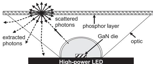
**Figure 4** Schematic of the SPE white LED package. (Not drawn to scale.)
