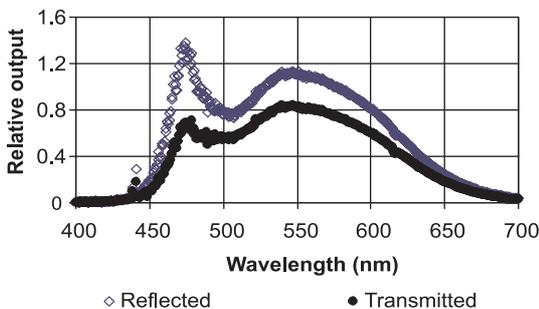
**Figure 2** (online colour at: www.pss-rapid.com) Spectral power distributions for the transmitted and reflected radiations of one phosphor-coated plate (7 mg/cm<sup>2</sup>).
