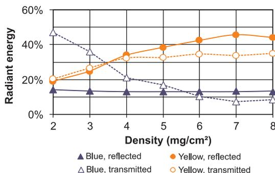
**Figure 3** (online colour at: www.pss-rapid.com) Transmitted and reflected radiant energies for blue and yellow light, as a function of phosphor density.
