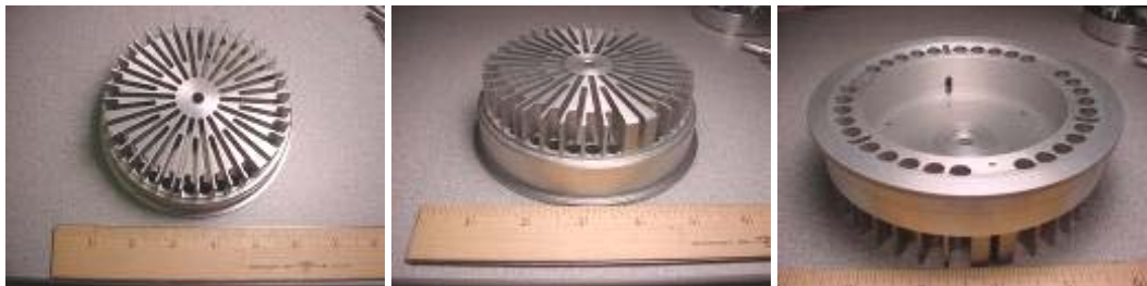
Figure 20. Top, side, and bottom views of the LED heat sink.
