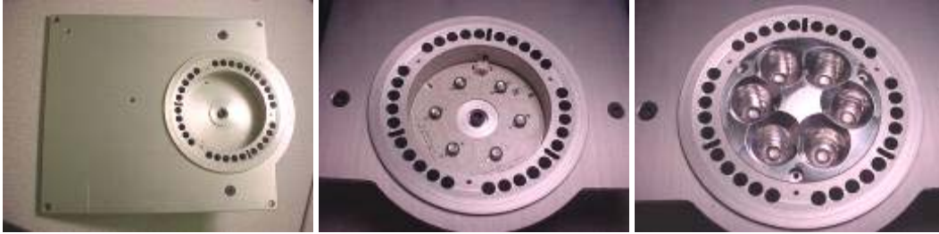
Figure 22. Bottom view of the mounting plate with LED heat sink in place (left), LED ring mounted to the heat sink (center), and bottom view of the complete fixture (right).
