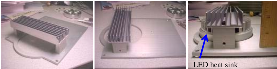
Figure 19. Mounting plate and additional heat sink (left and center), and side view with LED heat sink mounted in place (right). The additional heat sink was procured for the 5W LED assemblies and was not planned to be used in the field evaluation of the 3W LED assemblies.
