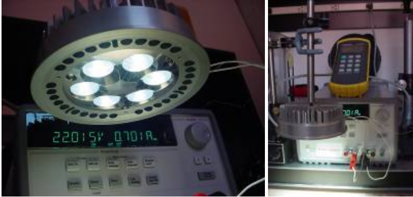
Figure 26. Bottom view of the heat sink and reflector with LEDs turned on during temperature measurement in open air.
