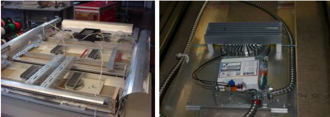
Figure 31. Top view of the ceiling panel built to house the low-profile LED luminaires for the field evaluation (left) and a close-up of one low-profile LED luminaire installed in the ceiling panel.
