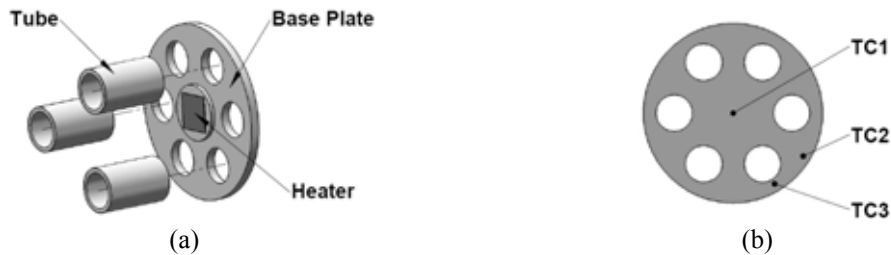
Fig. 4. (a) Exploded view of heat sink (b) Thermocouple locations (TC1-TC3) on the back of the heat sink
