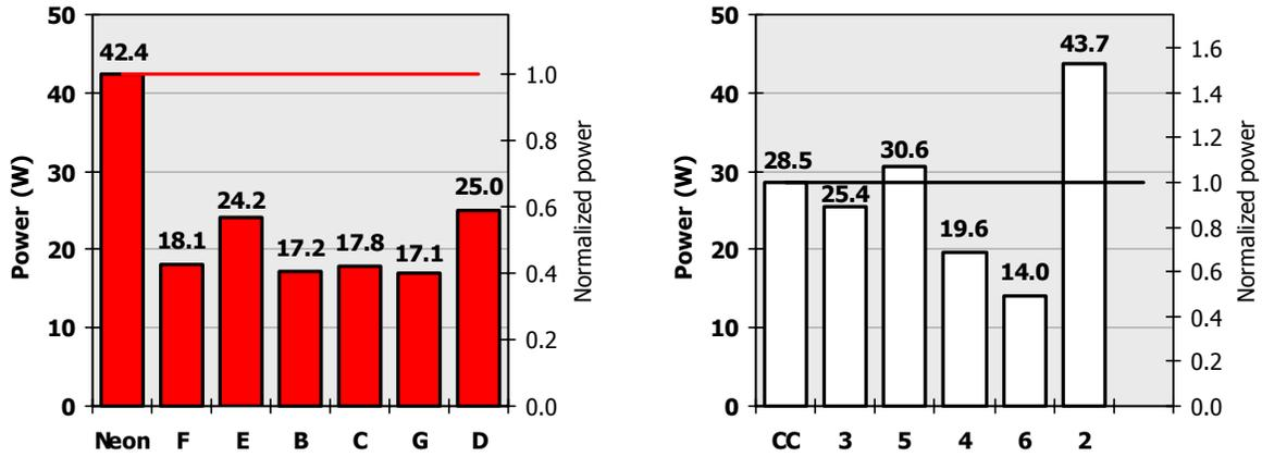
**Figure 3.** Measured power of all **RED** (left) and **WHITE** (right) signs tested. Each value is the average of five measurements at the end of the 90-minute stabilization period. The references for normalization (secondary axis) are the neon sign (for **RED**) and the cold-cathode sign (for **WHITE**).
