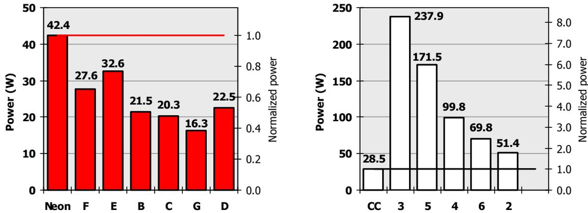
**Figure 4.** Scaled power of all LED signs for equal light output as the neon (for **RED**, left) and cold-cathode (for **WHITE**, right). The references for normalization (secondary axis) are the neon sign (for **RED**) and the cold-cathode sign (for **WHITE**).
