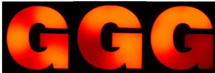
**Figure 6.** Reference conditions for each pattern: SPF1 (left), SPF2 (middle) and SPF3 (right). The contrast modulation value of these conditions was calculated at 0.70, 0.90 and 1.0, respectively.
