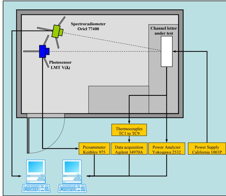
**Figure 1.** Schematic of the equipment used for the evaluation. Two computers collected the data systematically. The first controlled the spectroradiometer; the second controlled the LMT photosensor, the thermocouples, and the power analyzer.
