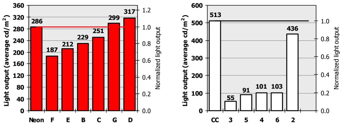
**Figure 2.** Measured light output of all **RED** (left) and **WHITE** (right) signs tested. Each value is the average of five measurements at the end of the 90-minute stabilization period. The references for normalization (secondary axis) are the neon sign (for **RED**) and the cold-cathode sign (for **WHITE**).
