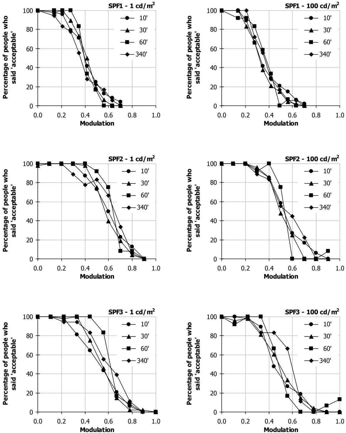
**Figure 7.** Acceptability rating (percent) for each condition, based on 48 answers from 16 subjects for patterns SPF1 (top), SPF2 (middle) and SPF3 (bottom) at four viewing distances (10', 30', 60', 340') for background luminances of 1 cd/m<sup>2</sup> (left) and 100 cd/m<sup>2</sup> (right).
