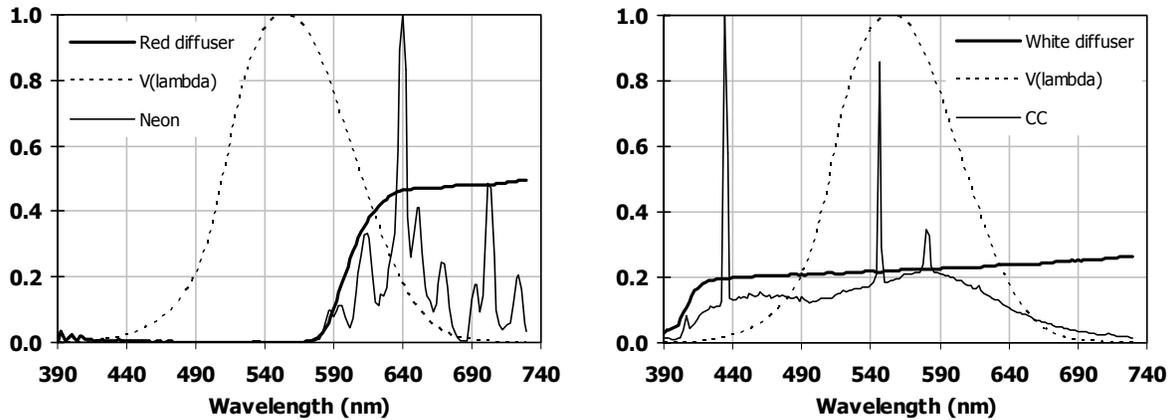
**Figure 5.** Relative spectral transmittance of the red (left) and white (right) acrylic diffusers, and spectral power distribution of the neon (left) and cold-cathode (right) lamps.
