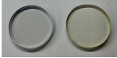
Figure 8. Picture showing the yellowing of the 3-mm sample after 560 hours.
