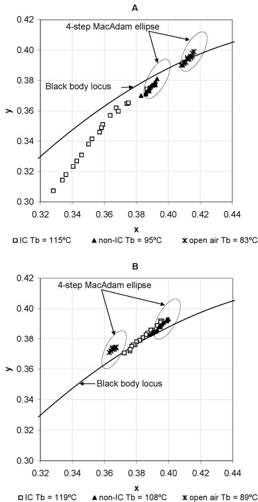
Fig. 6. Chromaticity values over time for the two commercial downlights tested in three application conditions.
