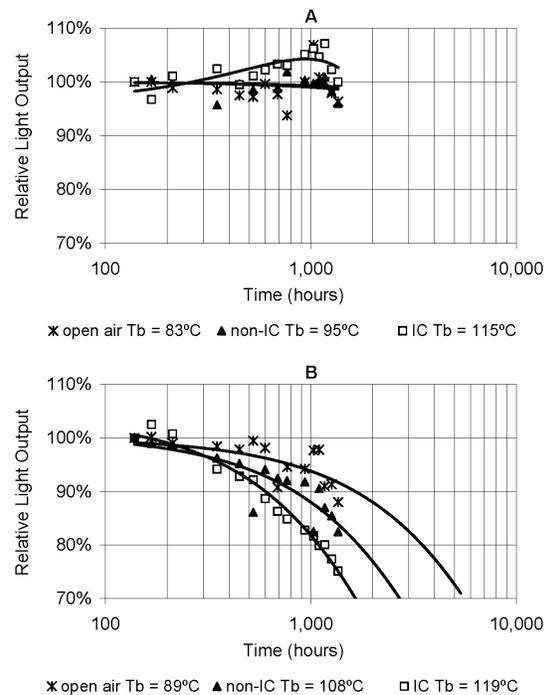
Fig. 5. Light output over time for the three environmental conditions for two 26-watt downlights.
