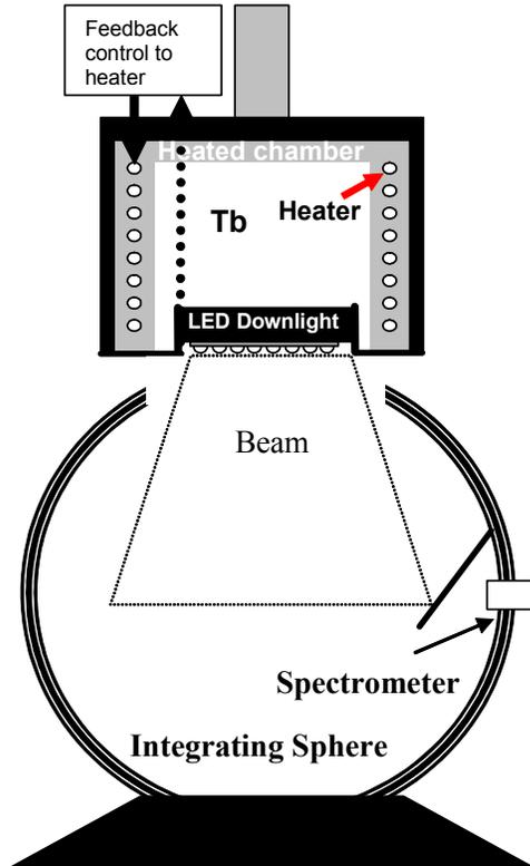
Fig. 3. Schematic of LED system life-test setup.
