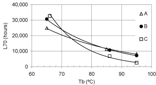
Fig. 2. Life, L70, as a function of board temperature for three LED groups.
