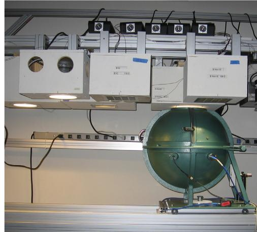
Fig. 4. LED fixture life-test setup.
