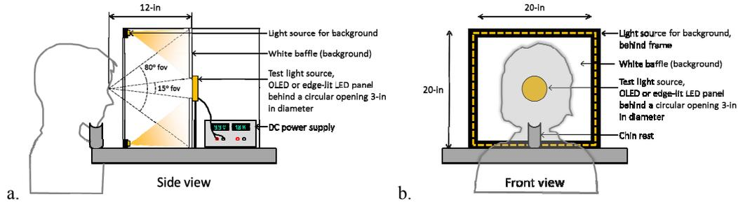
Figure 3. Illustration of the experimental setup: a) Side view; b) Front view (subject's view).
