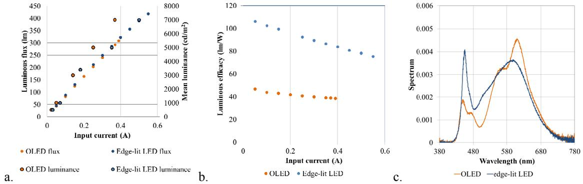
Figure 2. Photometric performance of the edge-lit LED and OLED panels used in this study, including a) luminance and luminous flux as a function of current; b) luminous efficacy as a function of current; and c) spectral power distribution.
