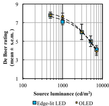
Figure 4. De Boer ratings (mean  $\pm$  s.e.m.) as a function of light source luminance for background luminance of 75  $\text{cd/m}^2$  and its corresponding illuminance at the eye of 100 lx.
