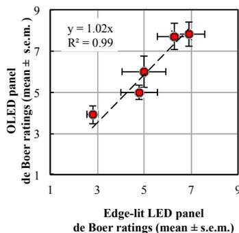
Figure 5. Correlation between the mean de Boer ratings of the tested conditions between OLED and edge-lit LED panels.
