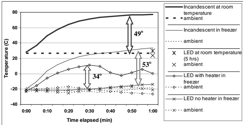
Figure 1. Fixture optics temperature over time.<sup>1</sup>
