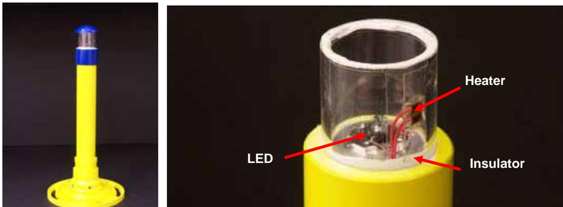
Figure 2. Solution 1 and its optics assembly.
