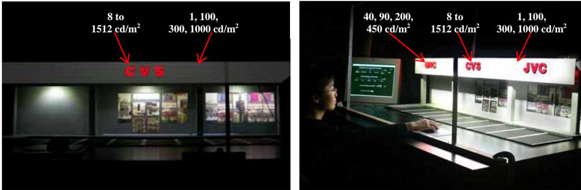
Fig. 1. Pictures of the scale model used for the subjective evaluations of signage brightness. The picture on the left shows the subjects' view during the experiment at a scaled 30-ft distance. The picture on the right shows the test sign amid two competing signs.
