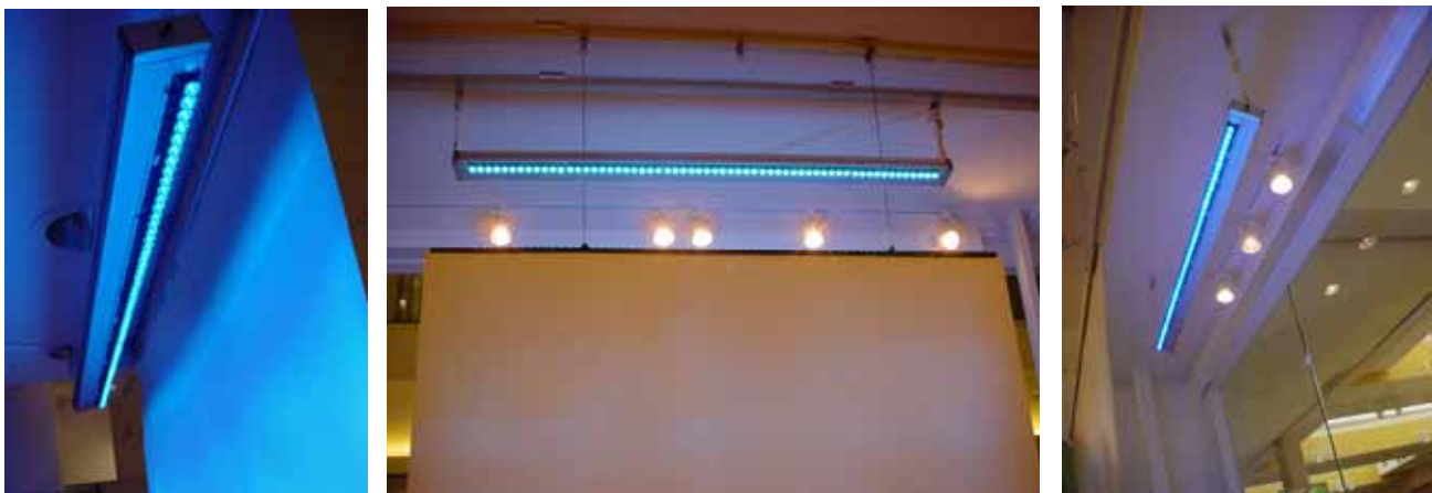
Fig. 2. Custom LED luminaires built for the study. The luminaires were hung from the ceiling or existing aluminum tracks used for poster displays. The distance to the poster ranged from 12 to 18 inches.
