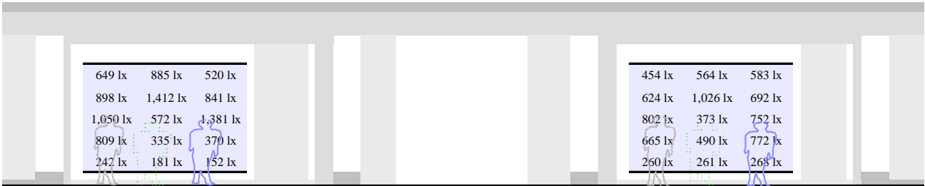
Fig. 4. The typical grid of vertical illuminance and luminance measurements taken for each window (Store 3, lighting condition 1 in this example). The top two rows indicate measurements on the background (i.e., blue illumination), whereas the lower three rows indicate measurements on the mannequins (i.e., accent lighting).
