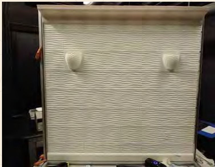
Figure 1. Prototype, scale-model sized 3D-printed wall with integrated lighting created at the Lighting Research Center.
