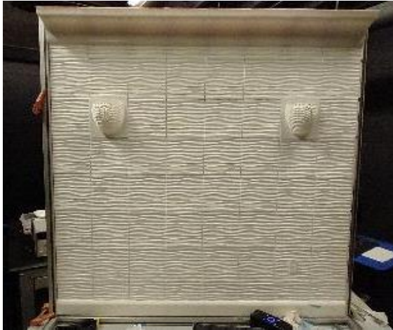
Fig. 1. (left) Prototype, scale-model sized 3D-printed interior wall with lighting (LRC photo) [11]
