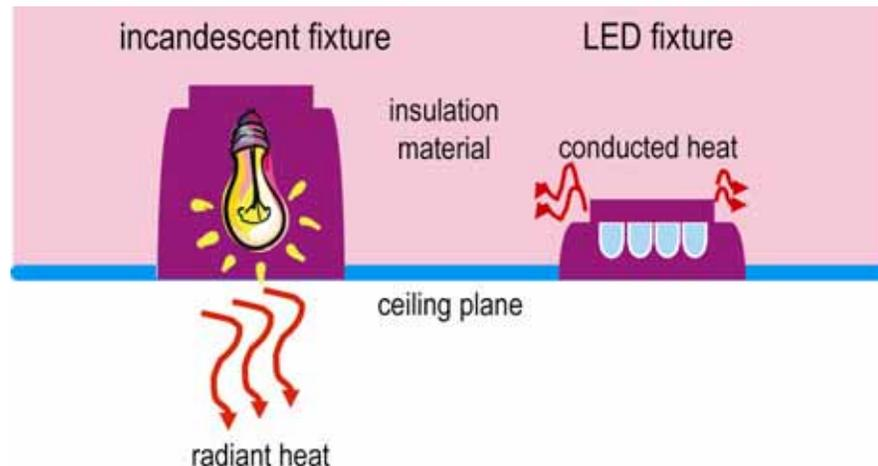
Heat transfer for an incandescent fixture and an LED fixture.
