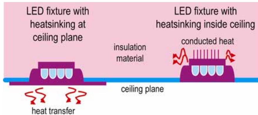
Heat transfer for two LED fixtures with different heat sinking options.
