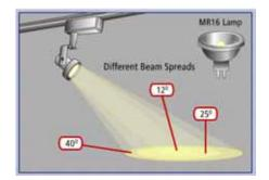
Examples of beam angles or beam spreads available for an MR16 lamp.
