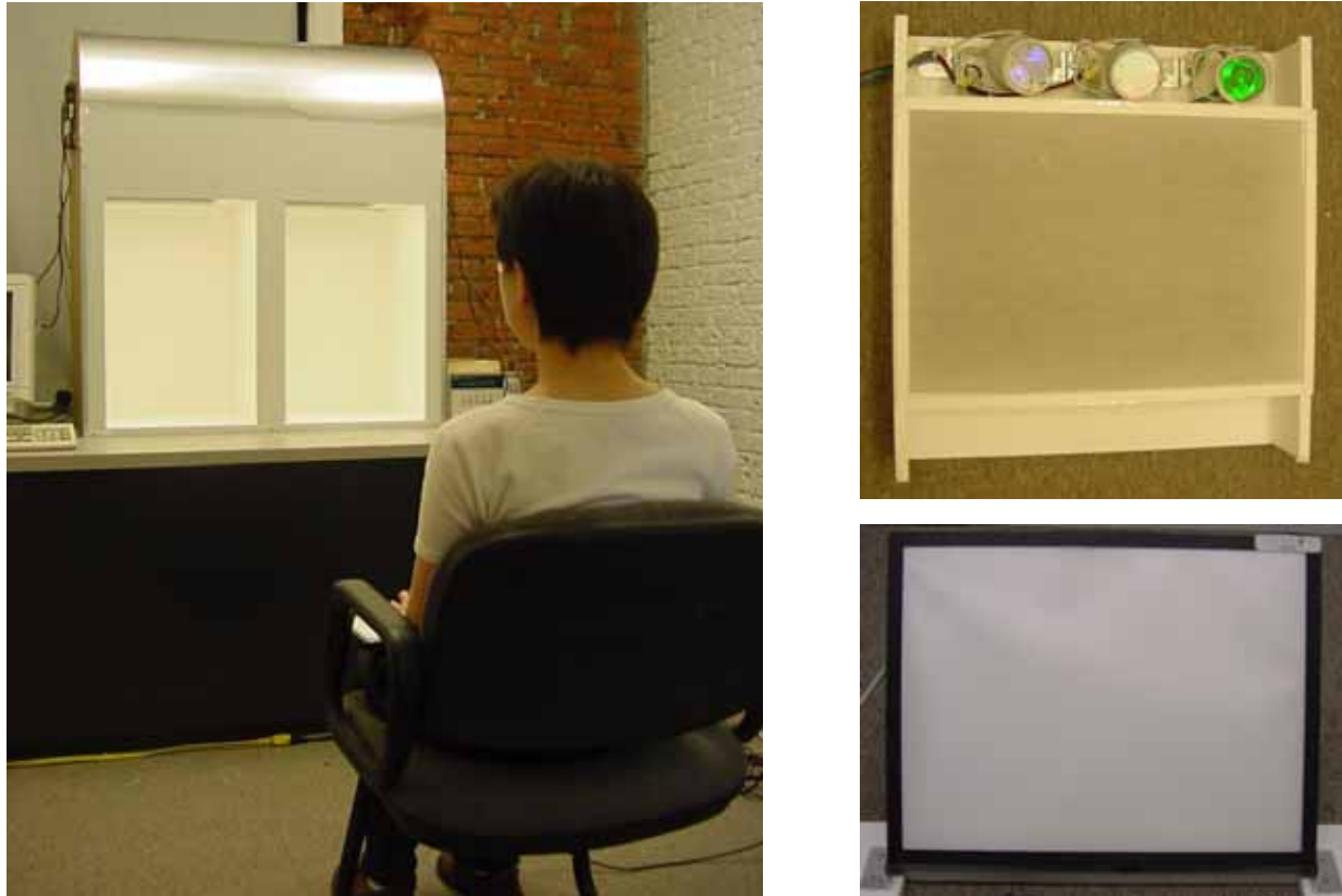
Figure 3: Subject looking at the experimental display cabinet (left); MR16 RGB mixed light system and diffuser (top right); RGB LED panel (bottom right).
