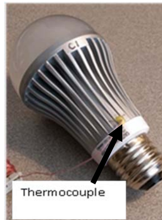
Fig. 3: Example of a thermocouple attached to the body of the LED A-lamp
