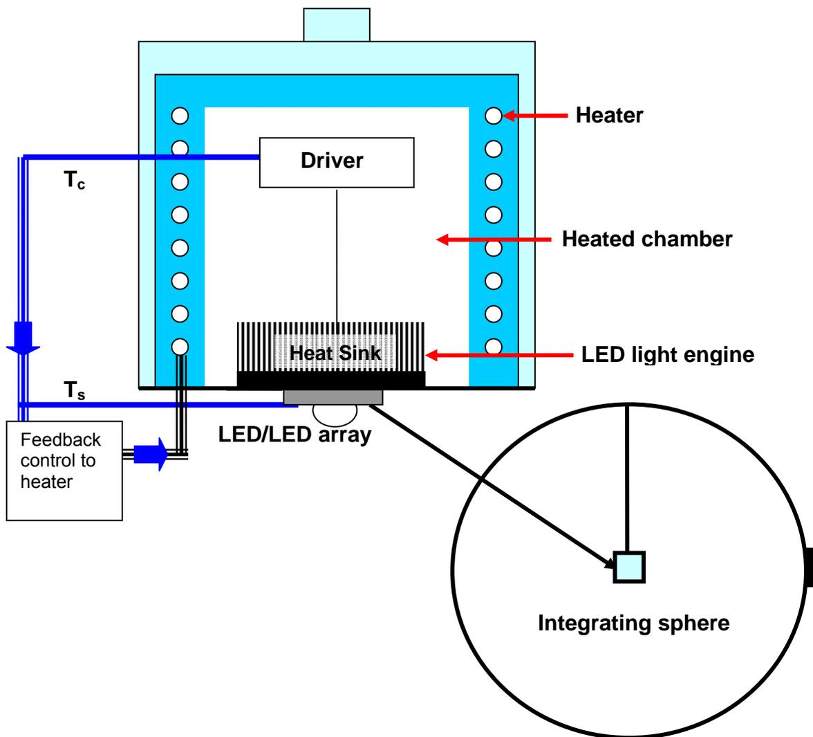
Figure B1. Schematic of the proposed test enclosure for sphere measurements.
