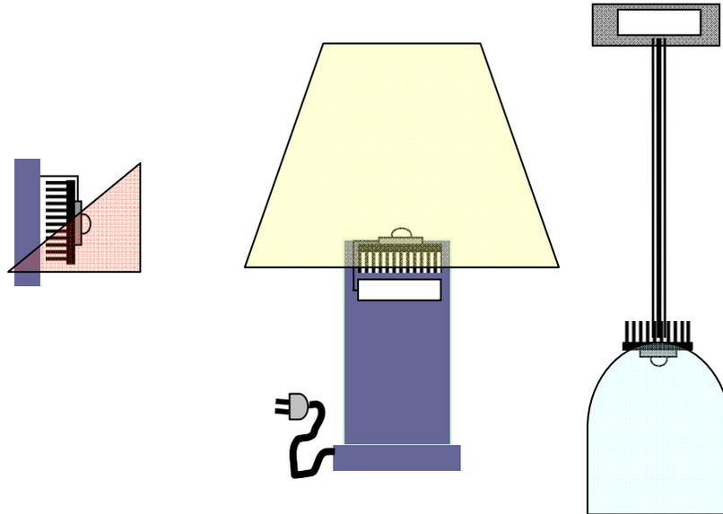
Figure 3. Examples of three different styles of luminaires incorporating the same LED light engine/lamp.
