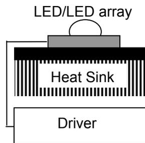
Figure 1. Example of an LED light engine.
