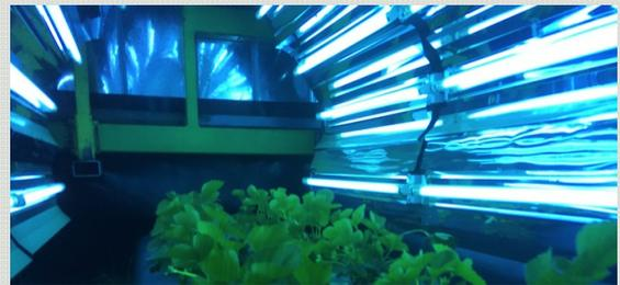
*Testing of tractor towed lighting apparatus for control of powdery mildew of strawberry.*
